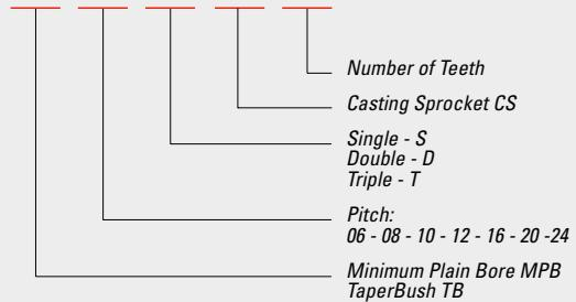
Casting Sprockets are made from EN-GJL-200 (GG20) according Standard EN-1561. See page number M4.
