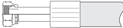
Female threads, DIN, BSP, OFS. Measuring reference point is the tip of the sealing head.
