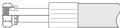
Female threads, DIN, BSP, OFS. Measuring reference point is the tip of the sealing head.
