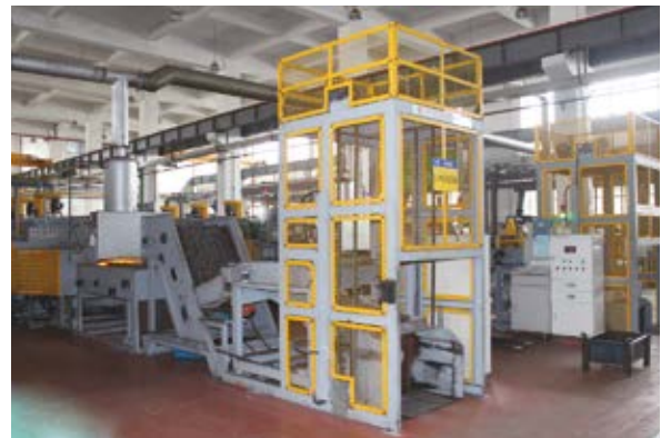
Continuous meshbelt furnace
