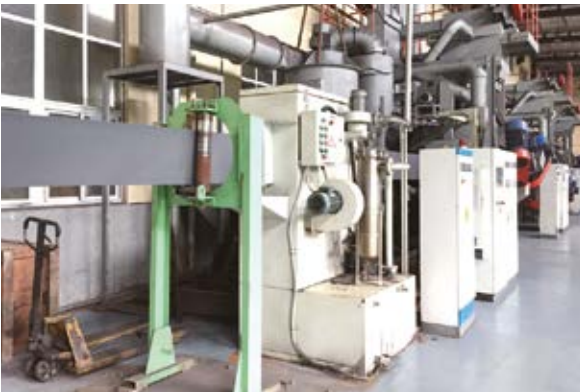
Environmentally friendly shot blasting line for plate material
