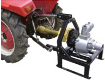
Tractor with a Water pump
