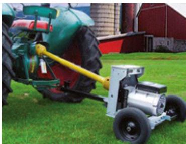
Tractor with an AC Generator
